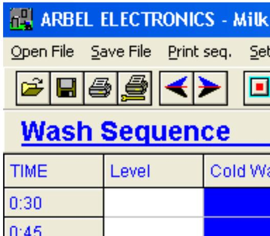
Once the wash sequence has been selected and modified in any way, it can be saved into the control system by clicking on the right facing arrow.
