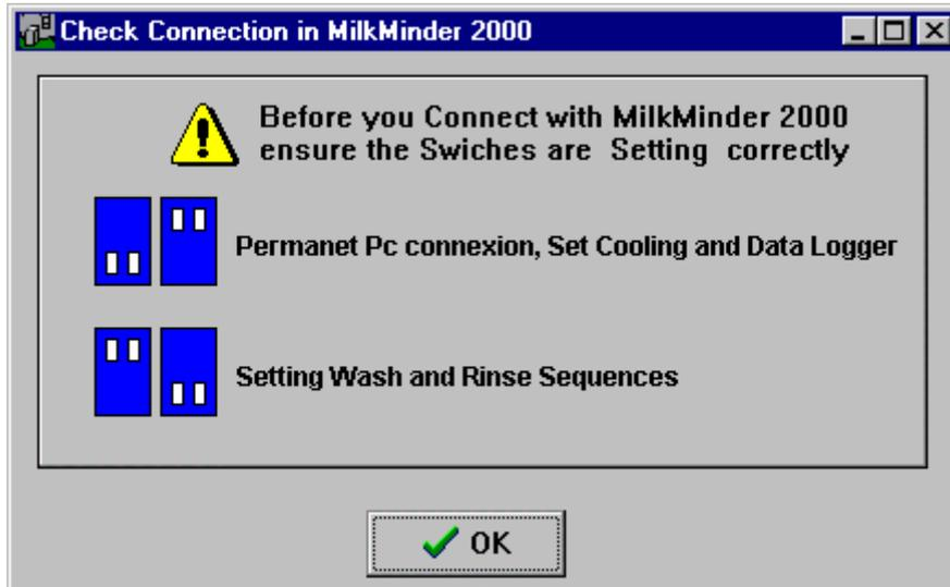
This screen is to remind you to set the DIL switches into the correct positions, depending on whether you want to view the cooling settings and data logger or the wash and rinse sequences.
